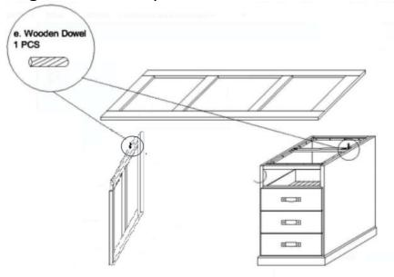
STEP 2: Carefully lift the pedestal upside down on the desk top and ensure the dowels sit firmly over the holes.
