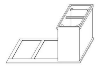
STEP 3:Put furniture connector on both side of the front rail,Fasten the front rail ③to the pedestal② with the allen bolt(b).
