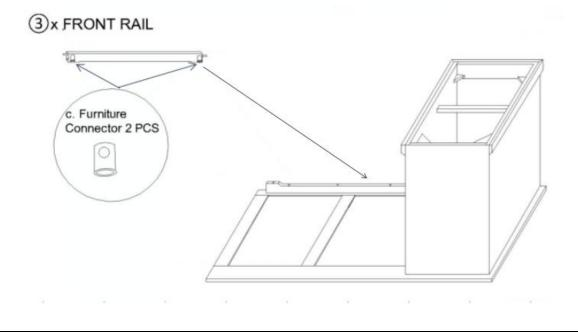
STEP 4: Flip the gable 4 upside down on the desk top 1 carefully. Fasten the gable 4 to the front rail 3 with allen bolt (b). Put furniture connector on both side of the back rail, Fasten the back rail 5 to the pedestal 2 and the gable 4 with the allen bolts(b).
